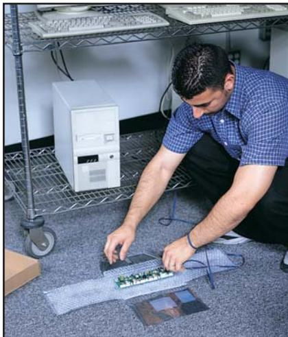
Attached to package is grounding strap with loop on one end to be snugly attached to worker's wrist. Other end has alligator clip to use to ground both worksurface and worker.
