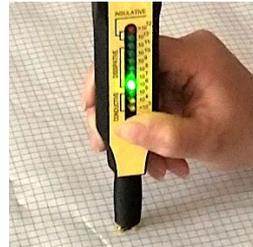
5. Read the Surface Resistance Range on the body of the probe.
