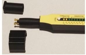
2. Point the two Pogo Pin Probe onto the surface of the material to be tested. Orient the Probe perpendicularly to the surface to be tested.
