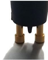
3. Push down on the probe until the probe limiter makes contact with the test surface.
