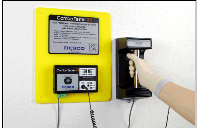
Figure 6. Using the ESD Glove Test Fixture with the Combo Tester X3
