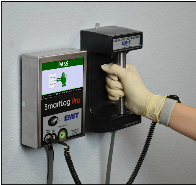
Figure 5. Using the ESD Glove Test Fixture with the SmartLog Pro®
