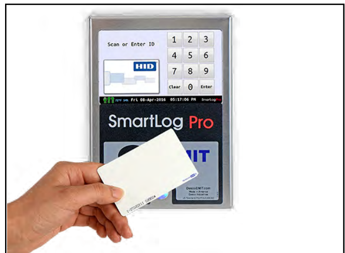
Figure 4. Holding a proximity badge in front of the RFID icon on the SmartLog Pro®
