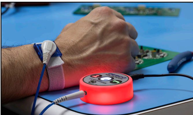
Figure 10. Illuminating red to indicate a broken operator path-to-ground
