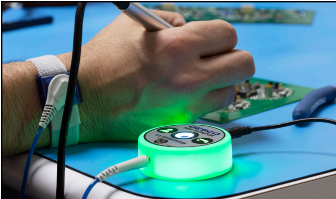
Figure 9. Illuminating green to indicate a proper operator path-to-ground
