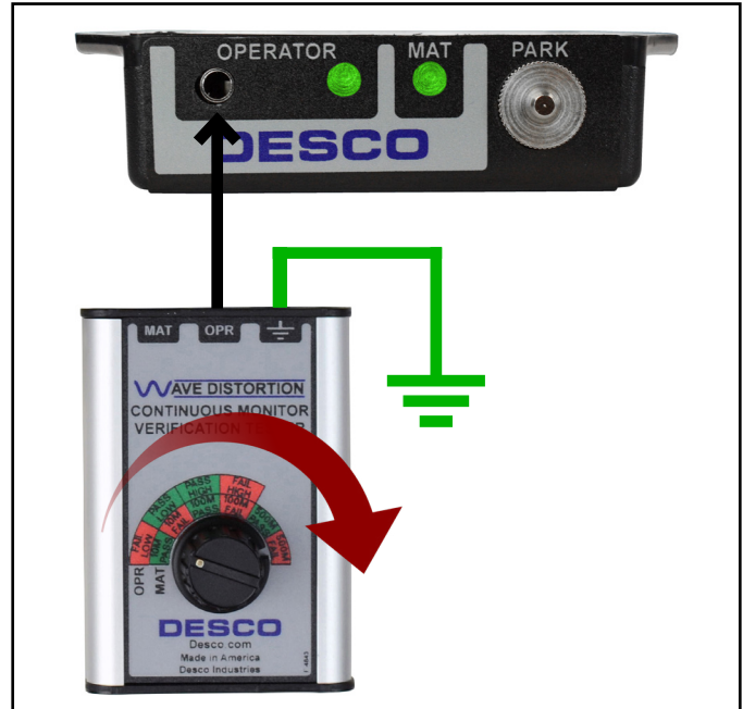
Figure 6. Connecting the Wave Distortion Monitor Verification Tester to the Multi-Mount Monitor's operator jack
