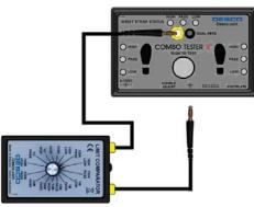
Figure 2. Wrist Strap Test Setup
