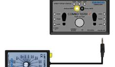
Set the knob on model 19254 to "750K Pass", touch the TEST contact on the tester and you should get a green LED for the left and right of the foot.
