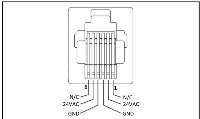
Figure 8. Pin-out of the console's power socket
