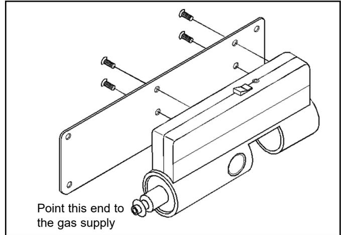
Figure 2. Securing the console to the mounting plate
