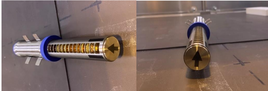
Figure 5.1 Illustrates the arrow on the sensor. In this instance, the ionizing source is directly above the Ionmaster therefore the arrow is faced upward
