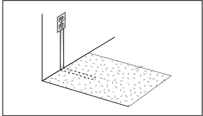
Figure 7. Properly grounding copper ground strips.
