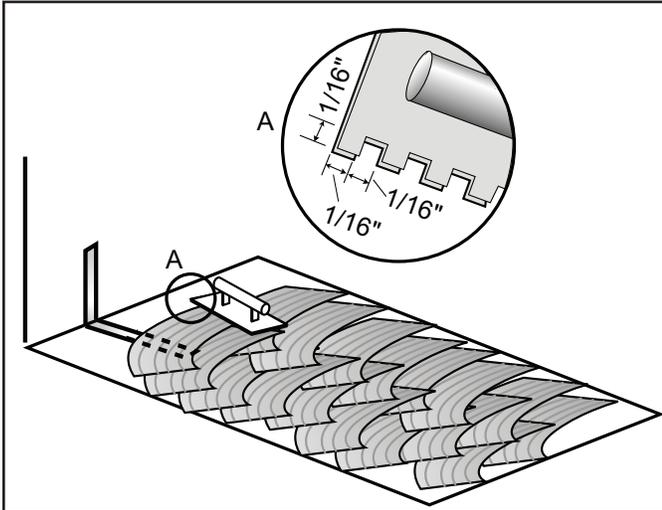
Figure 6. Spreading [8453](#) Conductive Floor Tile Adhesive.
