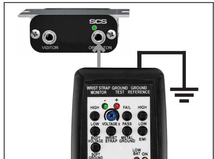
Figure 9. Connecting the Verification Tester to the WS Aware Monitor's operator jack
