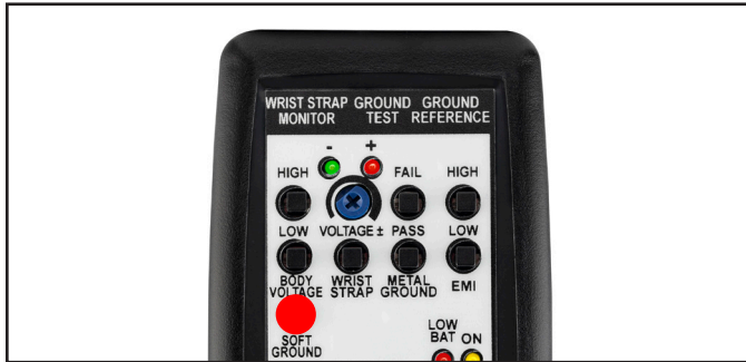
Figure 8. Pressing the SOFT GROUND test switch
