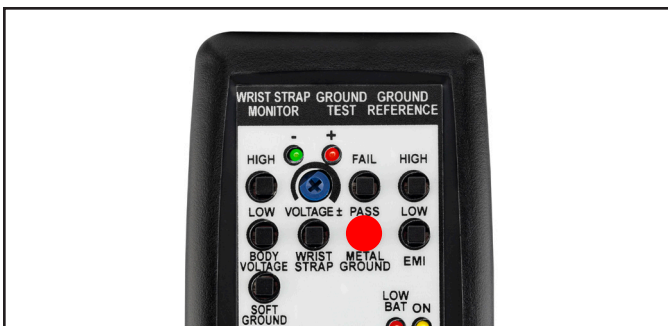
Figure 21. Pressing the METAL GROUND PASS test switch
