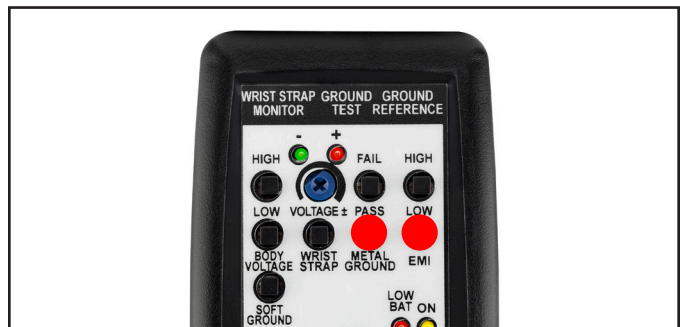
Figure 23. Pressing the METAL GROUND PASS and EMI LOW test switches simultaneously
