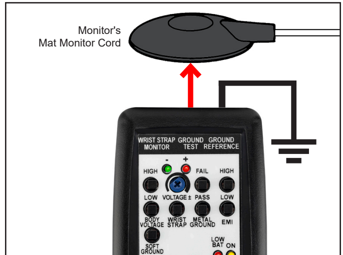
Figure 7. Connecting the Verification Tester to the Iron Man® Plus Workstation Monitor's mat monitor cord
