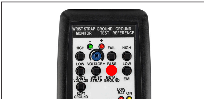
Figure 30. Pressing the METAL GROUND PASS test switch
