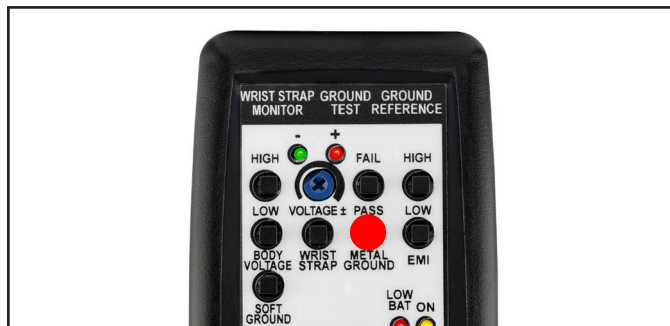
Figure 16. Pressing the METAL GROUND PASS test switch
