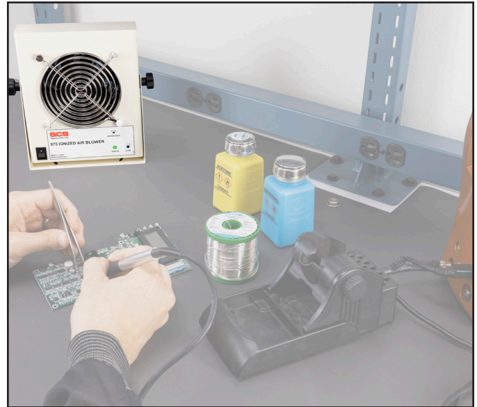
Figure 6. Using the 975 Ionized Air Blower on a workbench
