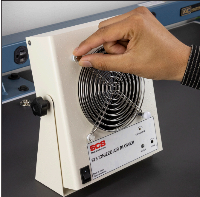
Figure 8. Loosening the fan grill thumbscrew
