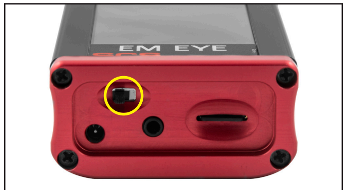
Figure 7. Location of the power switch at the bottom of the EM Eye Meter
