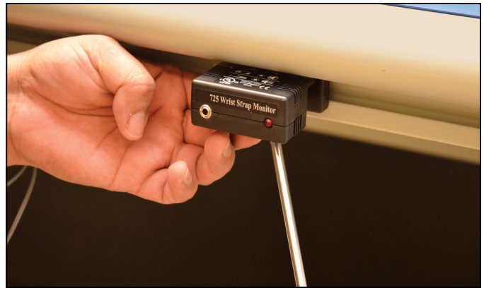
Figure 3. Installing the 725 Wrist Strap Monitor underneath a workbench
