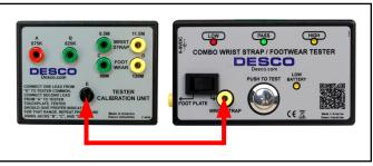
Figure 4. Connecting the test lead from banana jack "E" on the Calibration Unit to the WRIST STRAP banana jack on the Combo Tester
