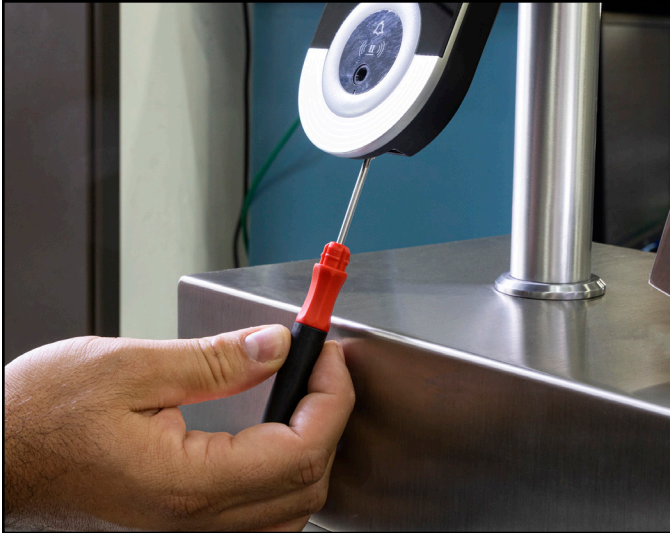
Figure 8. Securing the Facial Recognition Terminal to the back plate
