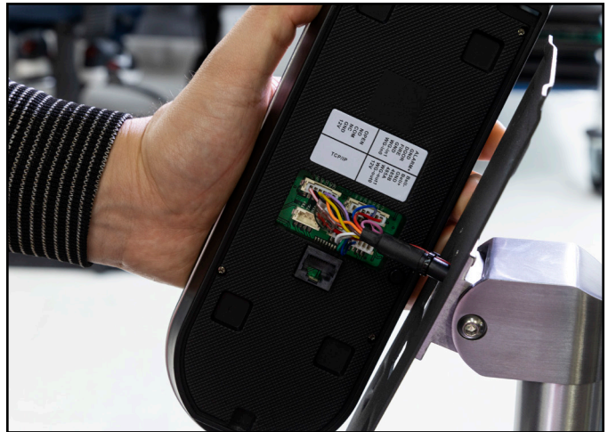
Figure 7. Connecting the wire harness to the Facial Recognition Terminal
