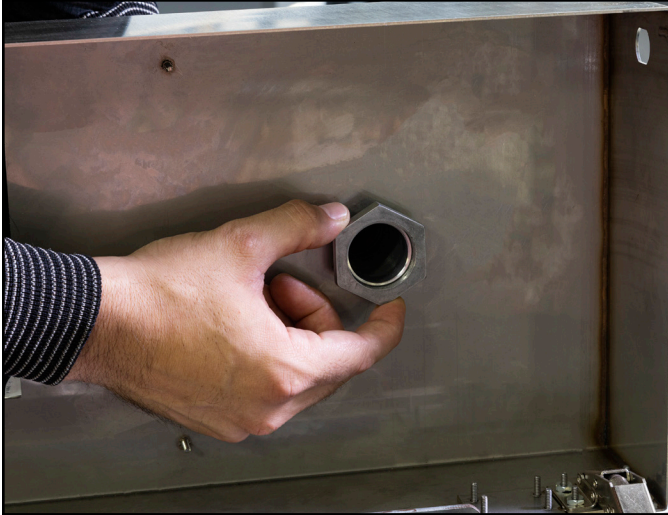
Figure 4. Using the nut to secure the mounting post onto the turnstile's lid
