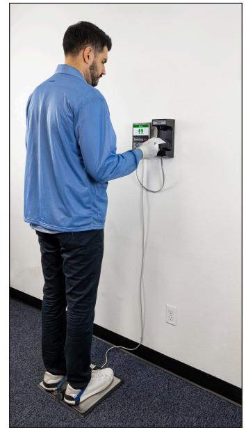
Figure 6. Using the Contactless Test Switch to perform a footwear test with the SmartLog Pro®
