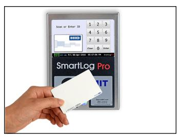
Figure 4. Holding a proximity badge in front of the RFID icon on the SmartLog Pro®
