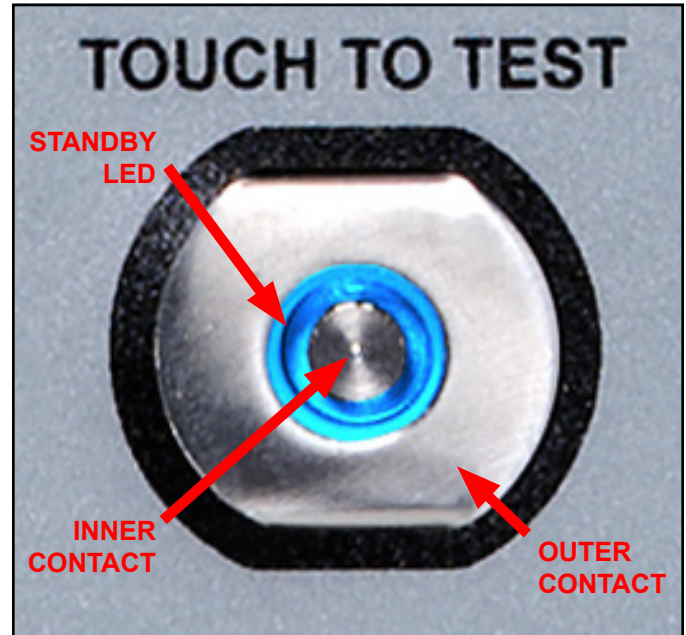
Figure 3. Steady-State Test Switch features and components
