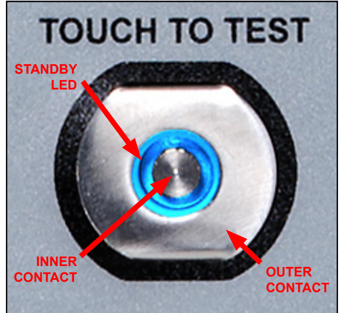
Figure 3. Steady-State Test Switch features and components
