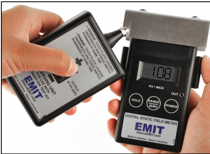
Figure 8. Taking decay measurements
