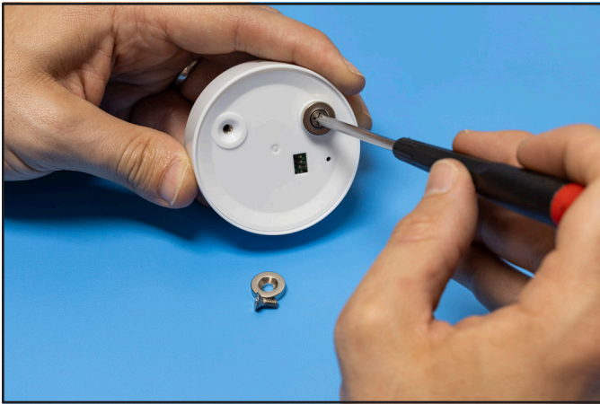
Figure 7. Installing the Desco 19344 Ring Magnets
