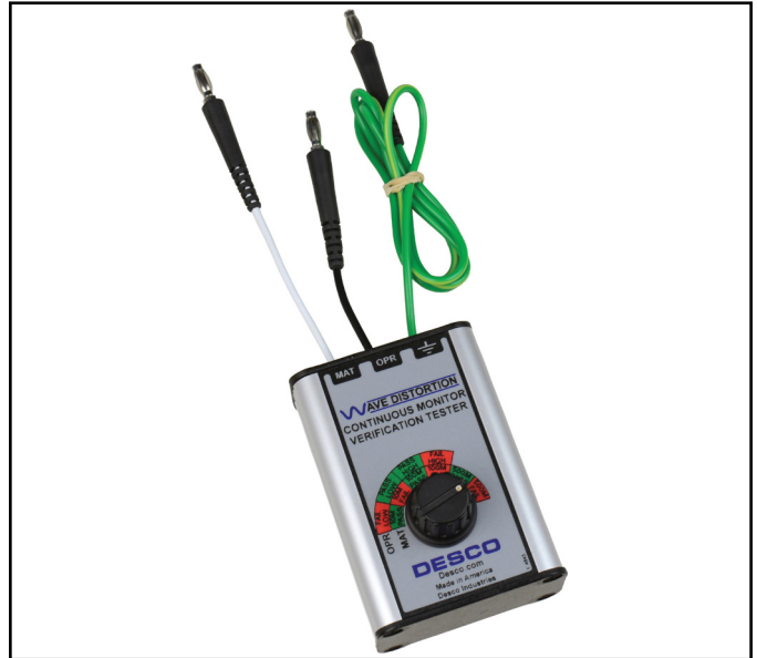
Figure 12. Desco 98221 Wave Distortion Monitor Verification Tester
