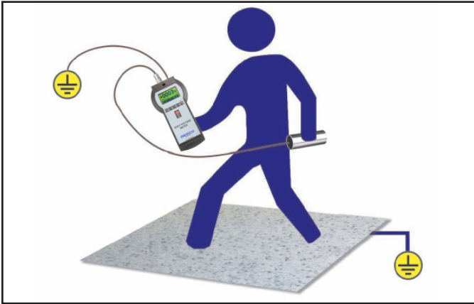
Figure 3. Setup of the Body Voltage Meter
