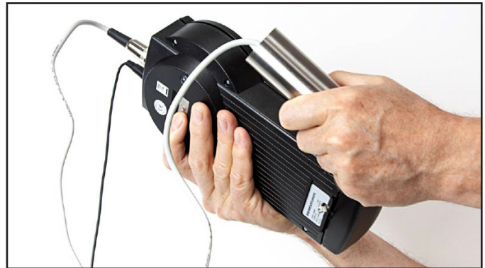
Figure 4. Touching the ground touch plate to ground the operator and zero the meter
