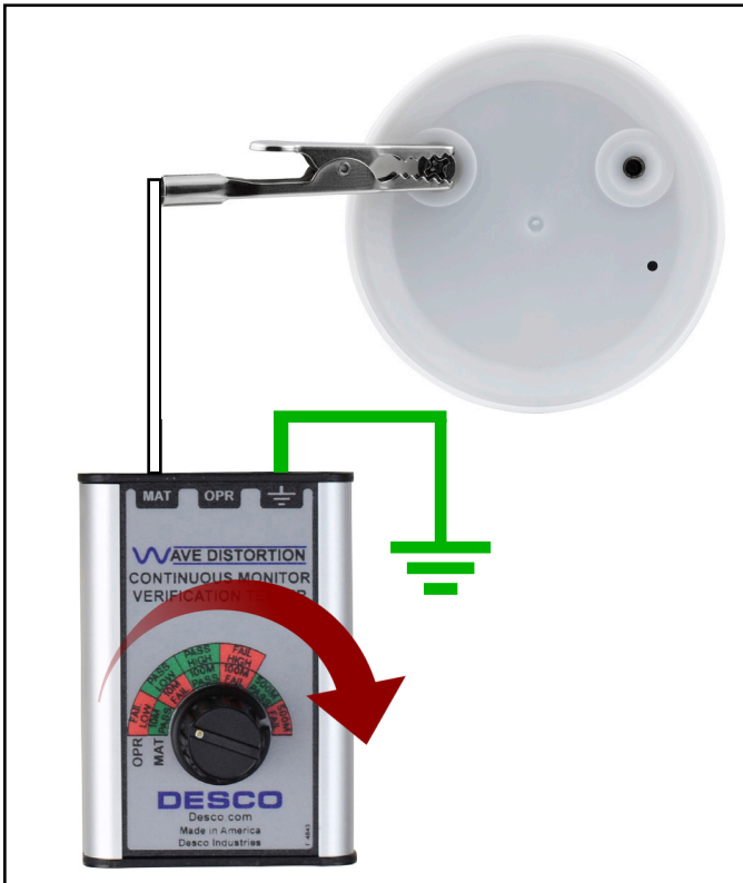
Figure 6. Using the alligator clip to connect the Wave Distortion Monitor Verification Tester to the Mini Monitor's worksurface monitor terminal
