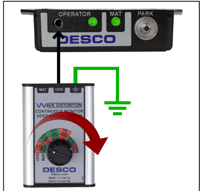
Figure 7. Connecting the Wave Distortion Monitor Verification Tester to the Mini Monitor's operator jack
