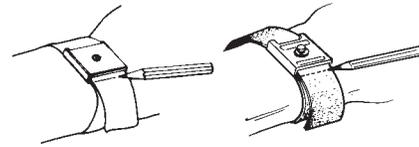
3. Tighten or loosen the elastic material through the clasp until the wristband fits snugly but comfortably.
