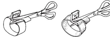
4. We recommend that you close the clasp and wear the band with the excess tail extended for a day to be sure the adjustment is snug, comfortable, and has the proper electrical contact with the skin before cutting.
