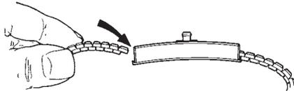
2. Change the size of the band by sliding the links in or out of the stainless steel backplate. For extra small users you can cut off excess links with cutters.
