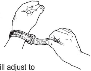
1. Attach wrist strap on wrist so that the black conductive band makes contact with skin.
