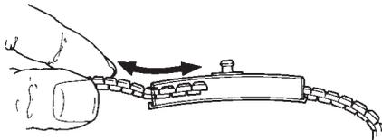
3. Lock the links into place by pulling down on the band, seating the band securely over the lip on the edge of the backplate.
