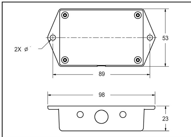
Figure 5. Mounting hole locations of the Satellite Remote (dimensions in mm)
