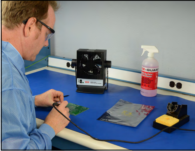
Figure 2. Using the 963E Benchtop Air Ionizer
