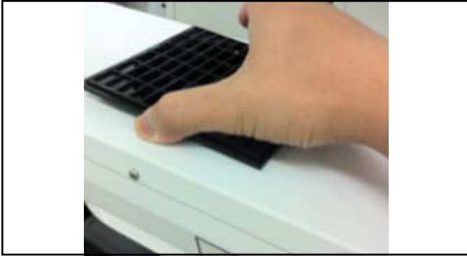
Figure 5. Remove the back grill by pressing the latch tabs on each side and pulling off
