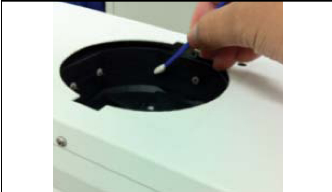
Figure 6. Wipe the emitter tips, brushes and fan blades with a cotton swab or brush. After cleaning, re-install the front grill.
