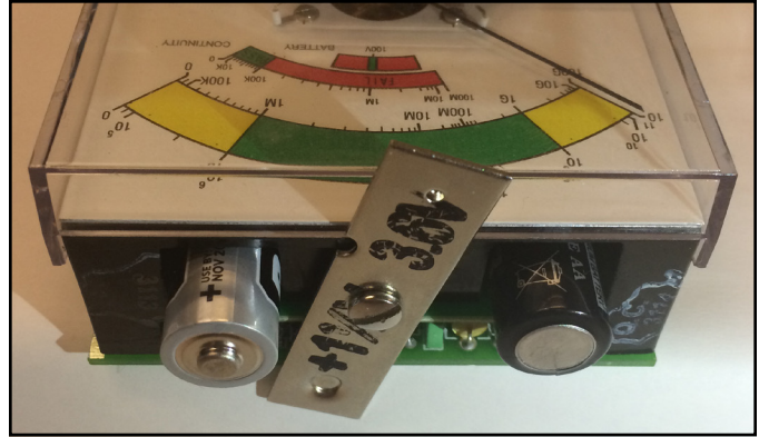
Figure 9. Replacing the batteries
