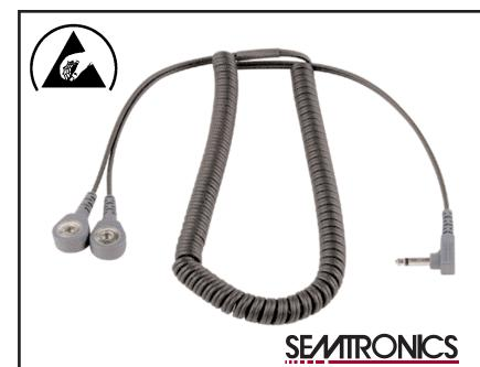
"If any part of the loop should open (become disconnected or have out of limit resistance), the circuit will go into the alarm state" [ref TR20.20], nonetheless, due to the redundancy inherent in the dual wire wrist strap design, the operator will continue to be grounded via the second intact wire.
