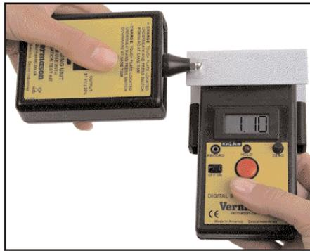
Figure 6. Taking decay measurements
