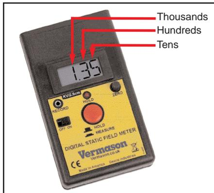
Figure 4. Reading the Digital Static Field Meter
