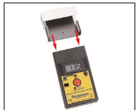
Figure 2. Installing the 222661 Conductive Plate
