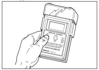
Figure 3. Zeroing the Fieldmeter
