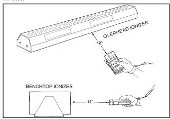
Figure 4. Taking a balance measurement.
