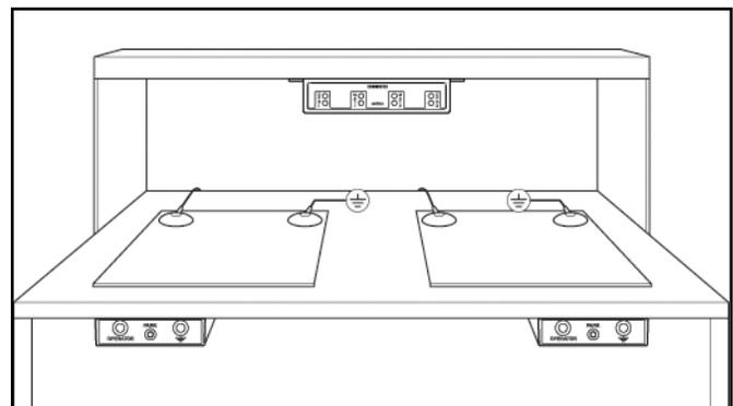
Figure 3. Typical setup of the Dual Operator Continuous Monitor and Satellites
