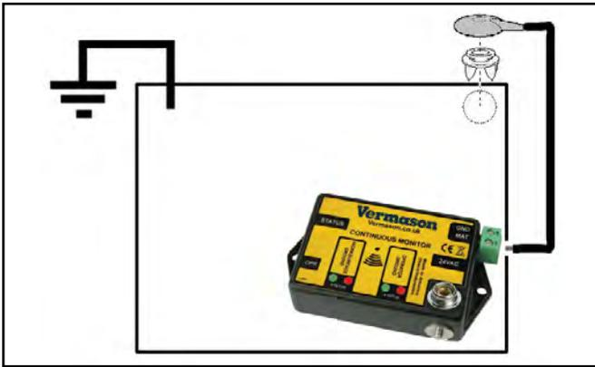
Figure 4. Installation method #2 of the Multi-Mount Continuous Monitor
