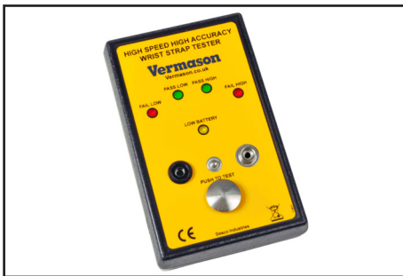
Figure 1. Vermason 222543 High Speed, High Accuracy Wrist Strap Tester
