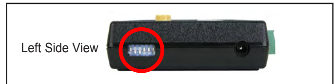
Figure 2. Locating the DIP switch on the Combo Tester X3
