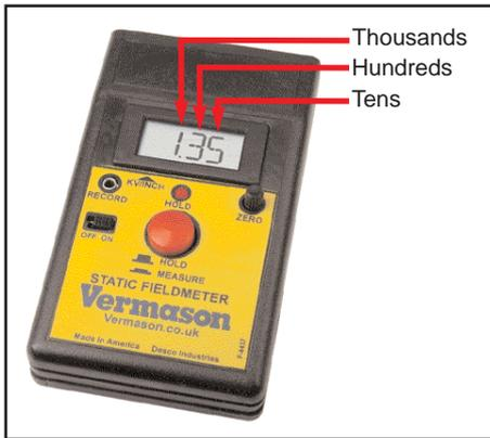
Figure 2. Reading the Digital Static Fieldmeter
