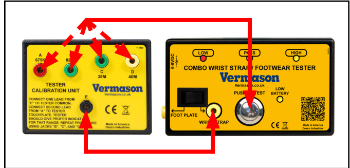
Figure 5. Verifying the calibration of the wrist strap circuit in the Combo Tester
