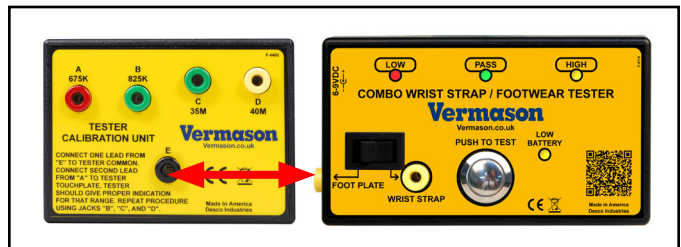
Figure 6. Connecting the test lead from banana jack “E” on the Calibration Unit to the FOOTPLATE banana jack on the Combo Tester
