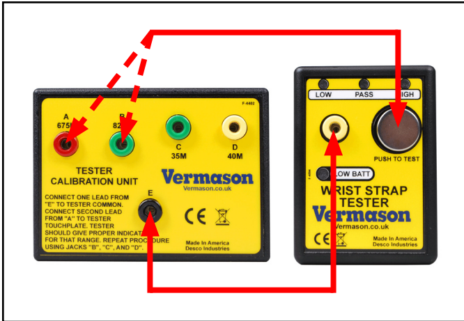
Figure 3. Verifying the low limit calibration of the Wrist Strap Tester
