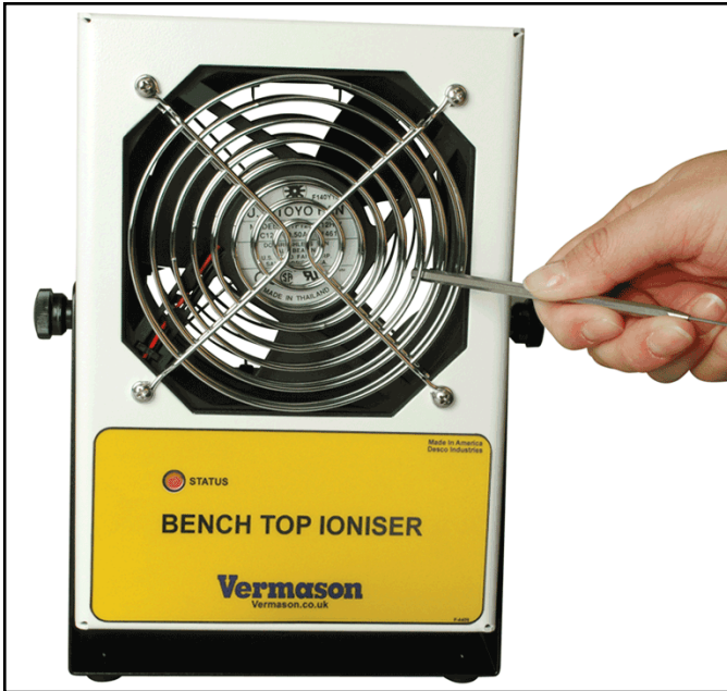
Figure 6. Shorting the ioniser's fan grills with a metal probe to test the alarm
