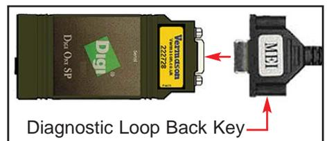
Figure 3. Connecting the Diagnostic Loop Back Key
