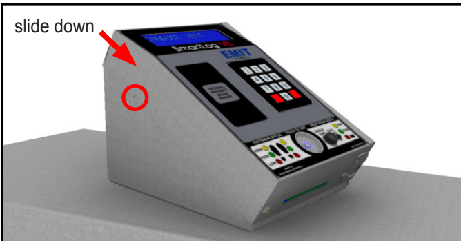
Figure 5. Sliding the SmartLog V5™ into the bracket and securing it into place with the 4-40 screw
