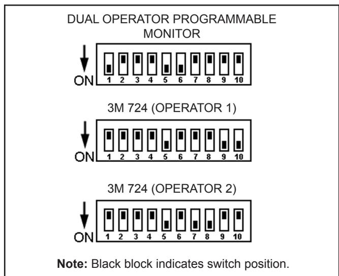
Figure 4. 50542 Universal Remote DIP switch settings
