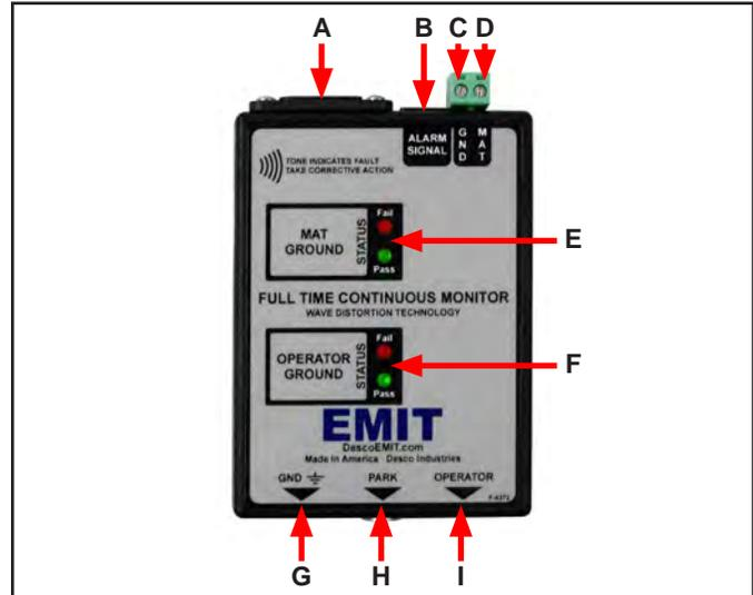
Figure 2. Full-Time Continuous Monitor features and components
