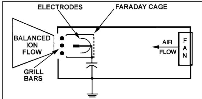
Figure 8. Components of the Faraday Balance System
