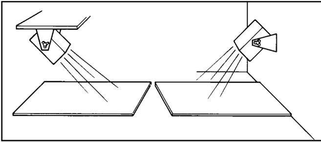
Figure 3. Wall or shelf mounting of the ionizer
