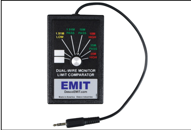
Figure 6. EMIT 50524 Limit Comparator for Dual-Wire Monitors
