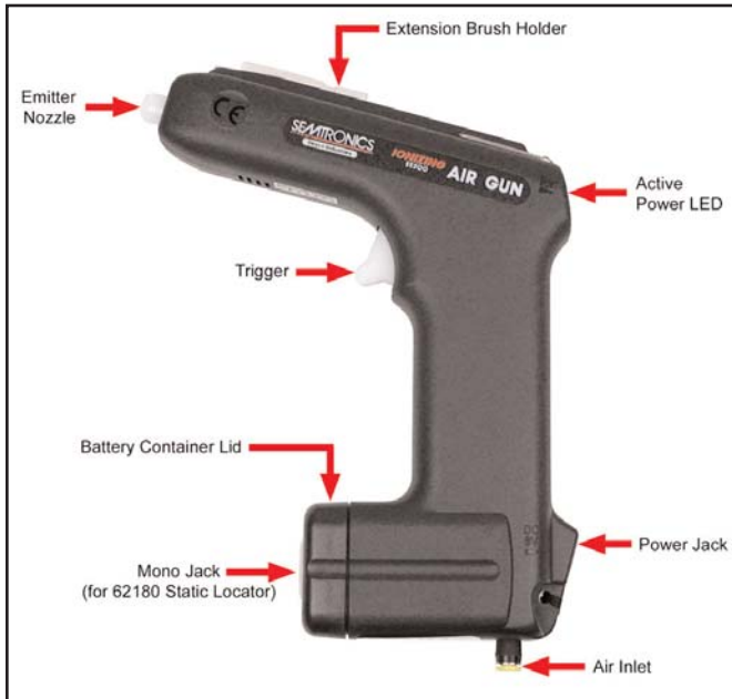
Figure 1. Ionizing Air Gun Features and Components
