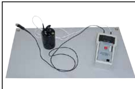
Figure 2. Testing RTG with Surface Resistance Test Kit.
