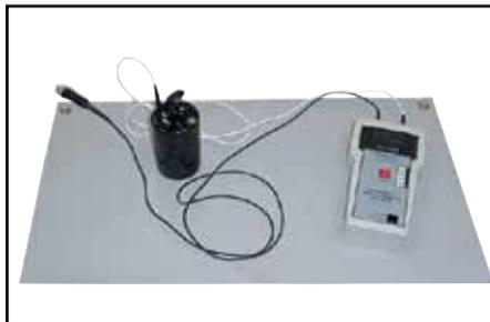
Figure 2. Testing RTG with Surface Resistance Test Kit.
