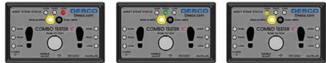
Wrist Strap Low Fail Wrist Strap Low and High Pass Wrist Strap High Fail
