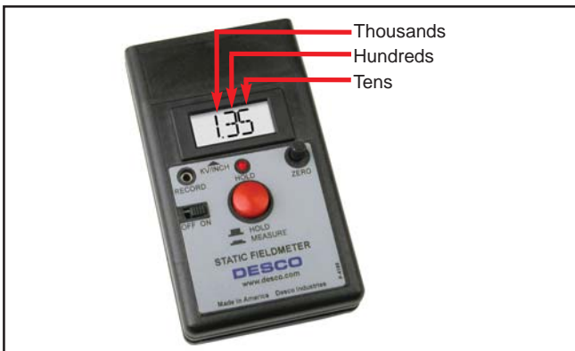
Figure 2. Reading the Digital Static Field Meter
