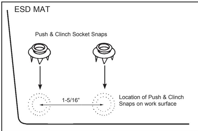
Figure 2. Installation of Push and Clinch Socket Snaps
