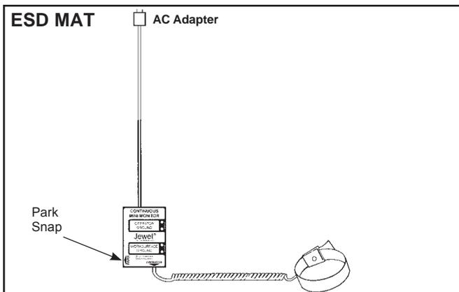
Figure 4. Jewel® Workstation Continuous Mini Monitor setup
