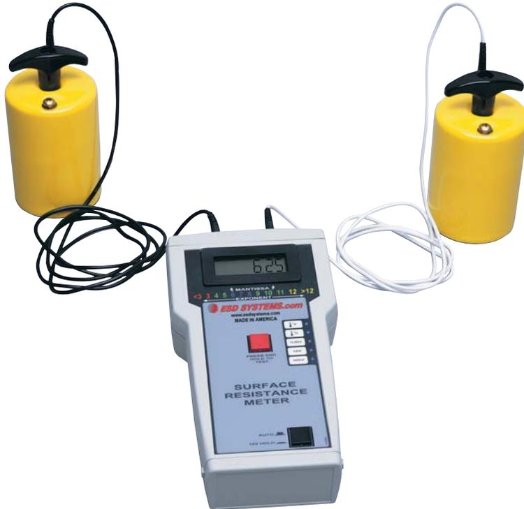
**Figure 1. Item 41290 Surface Resistance Test Kit**
