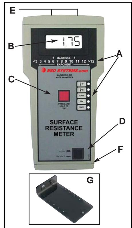
**Figure 2. Features of the Surface Resistance Meter**
