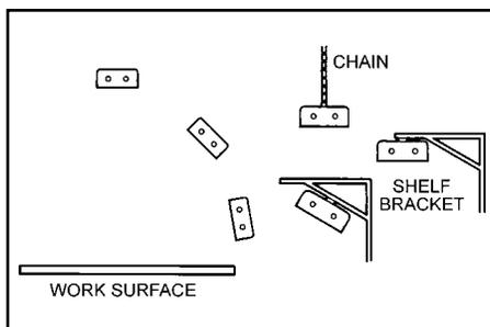
**Figure 3. Mounting alternatives relative to the bench top**
