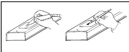
**Figure 6. Cleaning the emitters and fan guards**
